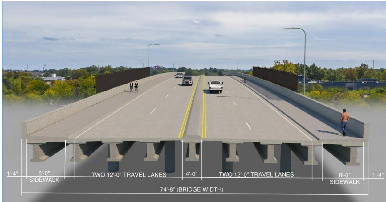
Figure 3. Bridge Typical Section.
